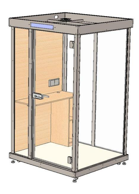
1. Fix Column A, Column B, Column C, and the door frame to the corresponding positions on the base using M6 $\times$ 20 countersunk screws, as shown in the diagram below.
