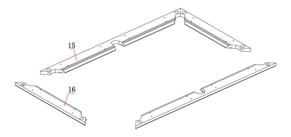
Attach side boards. (To avoid any damage, please layout some EPE foam or cardboard under the boards)
