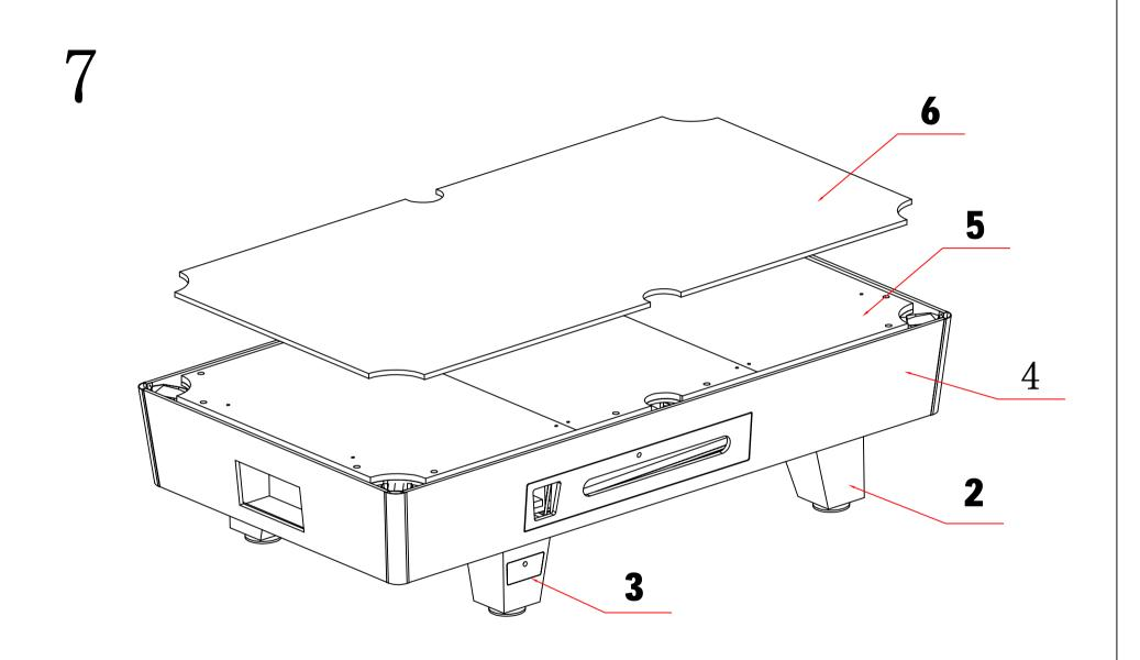
Secure the pool table cloth to the slate with stapler or glue
