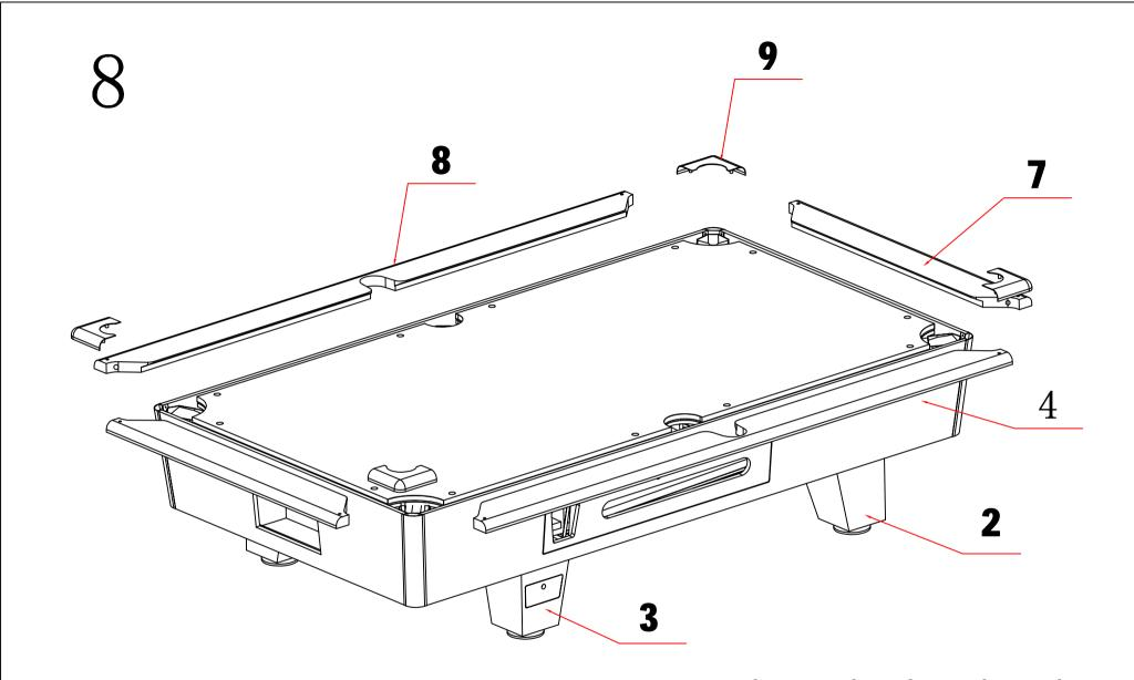
ut the end rails, side rails and table corner on the main structure as shown
