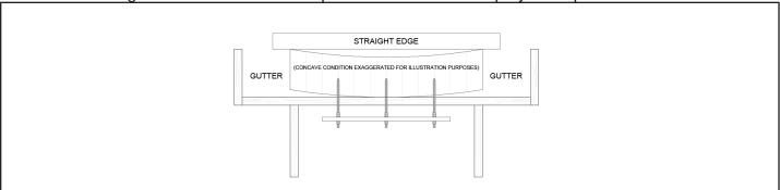
Important: nuts should be tightened slowly with 1/4 to 3/4 turns at a time. It may take a few days for the shuffleboard to completely react. DO NOT over tighten, as this can cause permanent damage to the Climatic Adjusters and your table.
