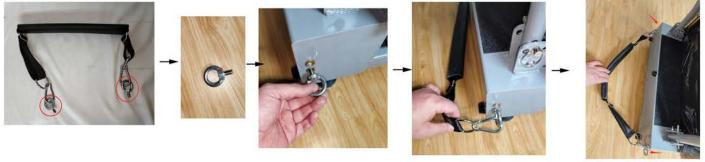
7.Loosen the plum screw, insert ③ into the round hole, and tighten the plum screw
