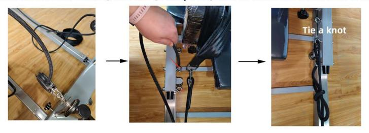
6.Remove the flange ring above the ⑤, screw it into the hole of the main body ①, and hang the ⑤
