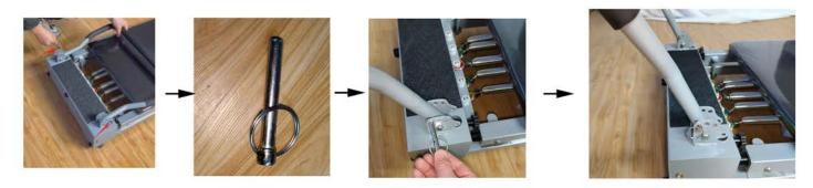
3. Loosen the plum screw, insert the 7, and tighten the plum screw
