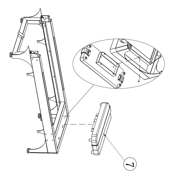
**Step 5**: The movable frame (9) is installed. Find the following accessories as shown in the figure below. All screws and screws are installed in a fixed position and can be installed after removing.
