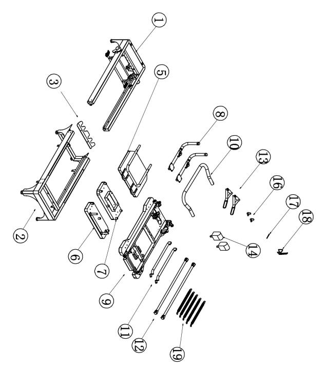
**Step 1:** remove the bubble pad wrapped on the mechanical parts, and then find out the following parts and install them according to the figure below;
