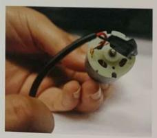
⑤Please using insul ating tape to twist positive and nega tive line to avoid the touch.
