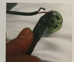
3Cut the positive and negative line from motor.
