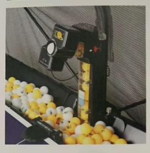
For prolonging its service life, ple ase use robot incl ean environment, clean the dust and wash the balls in certain time.
