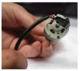
6 Please using insulating tape to twist the red and black line to avoid touching.
