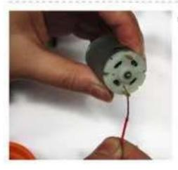
5 Prepare a new motor, connect the red line with the positive pole of motor, and the black line with its negative pole.
