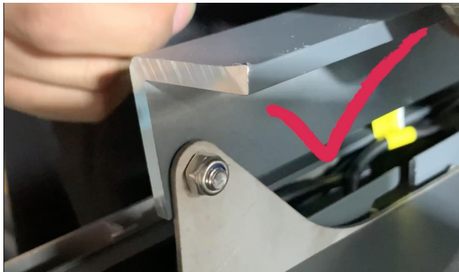
4, tightening only need to tighten the nut until you can not see the blue rubber ring, remember not to screw too tight, otherwise it will affect the flip of the louver
