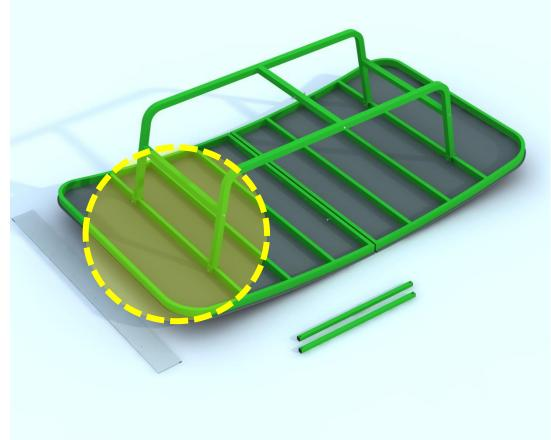
Connecting U Legs with Top A and Top B, Fasten the Screws
