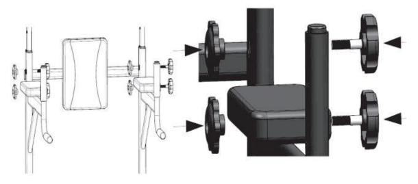
Step 11: Installing sit-up board
