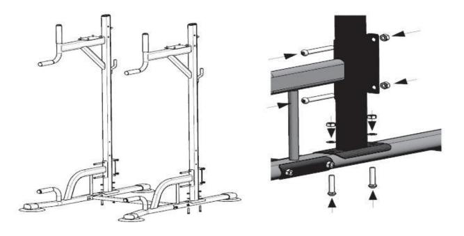
Step 5: Install the reinforcement tube
