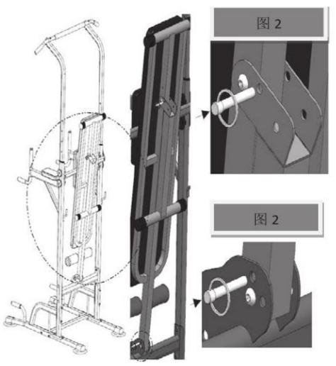
2. Pull out the supine plate fixing pin in the folded state. (Pay attention to holding the supine board.) Place the supine board down and level it to the ground.
