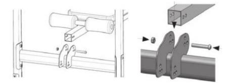
Step 12: Install the support plate of the supine plate
