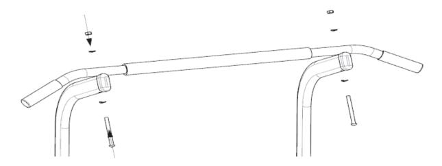
Step 10: Install the secondary pipe to adjust the height suitable for you
