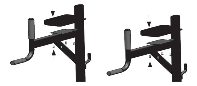
Step 7: Installing the back cushion
