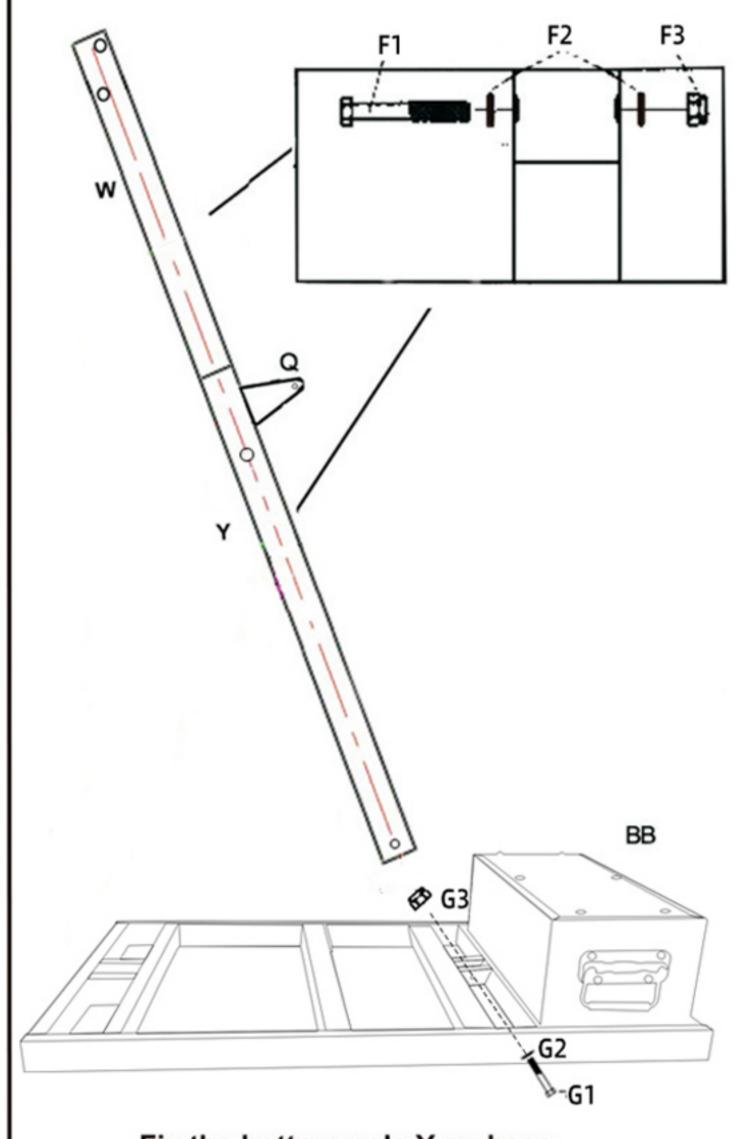
Fix the bottom pole Y on base BB by bolt G1. Make sure bracket Q face the back for next assemble step.
