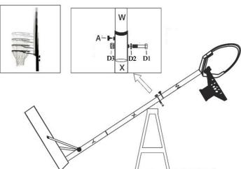
Insert the Top Pole(W) into Middle Pole (X),adjust it to required height, then fix them by Palstic Head Knob(A)&Bolt Set (D1),(D2)&(D3) as shown.Adjust the height by change the Bolt Set (D1),(D2)&(D3) in different holes on Top Pole(W).
