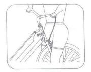
Check that the forks and the handlebars are facing forward and straight. Stand at the front of the handlebar, vise the front wheel by your legs and hold the handlebar, adjust the handlebar and the body of the bicycle to form an angle of 90degree, see the picture.
