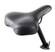
Your seat will tip forward for easy battery removal on most models.
